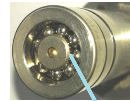
Ball bearing unit, lead coated balls
