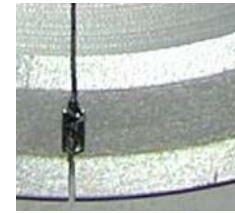
Anode crack (left), eroded focal spot track
