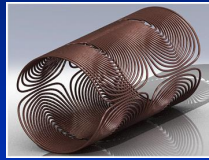
Schematic diagram of a gradient coil
