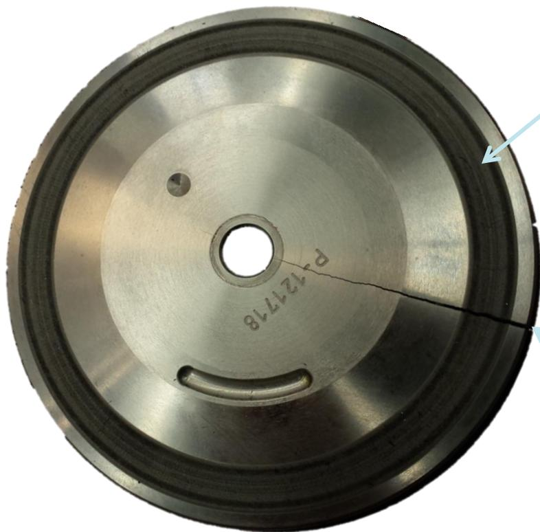
Focal track roughened during thermal cycling
