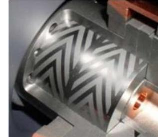
The two radial bearings of an SGB.
