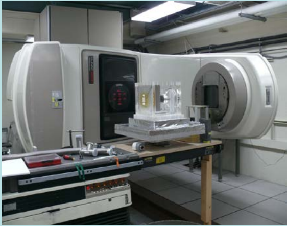
BIPM primary standard for clinical accelerator dosimetry
