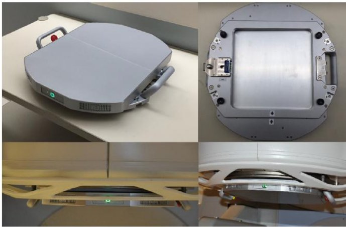
FIG. 1. The Integral Quality Monitor (IQM) is a large area ion chamber (top left) with a gradient of the ion chamber thickness in the axis of MLC motion. It attaches to the accessory tray holder, similar to an electron cone (top right). The device has a low profile from the linac head (bottom left and right) and connects wirelessly to a transceiver and the controlling computer.
