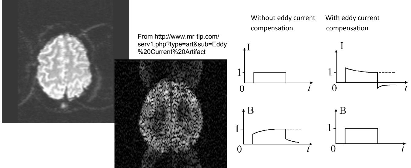
Eddy currents: Electrical currents running in the superstructure of the MRI can counteract the gradient fields. Occurs when the switching is fast and the gradients are strong (e.g., EPI, diffusion, etc)
