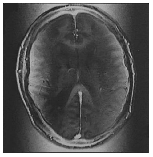
Pre-scan gain adjustment of receiver is too narrow to contain range of voltages observed in RF coil.
