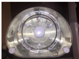
Figure 2-1: Cross Section of NEMA Image Quality Phantom (Demonstrating Proper Orientation of Hot and Cold Spheres)
