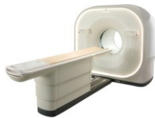
Philips Vereos PET/CT 20mm thick LYSO 1-1 coupling with digital SiPM TRes: 310ps
