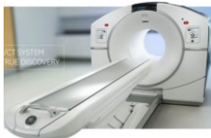
GE MI PET/CT 25mm thick Lu-based scintillator ~2-1 coupling with SiPM TRes: 390-400ps
