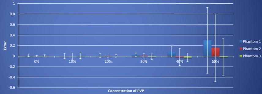
Error in measured ADC values in three different diffusion phantoms across the PVP concentrations in the phantom
