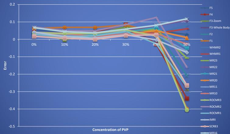
Error in measured ADC values in 20 different MR systems across the PVP concentration in the phantom
