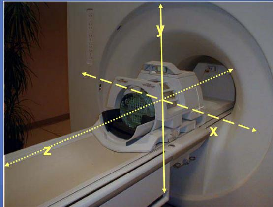
**Note: The slice, frequency and phase encoding may be on any axis!!!**
