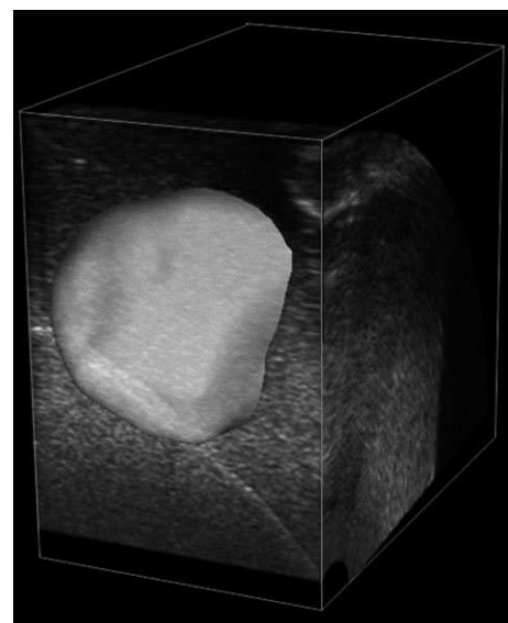
FIG. 5. 3D US image of the volumetric phantom showing the surface of the segmented tumor.
