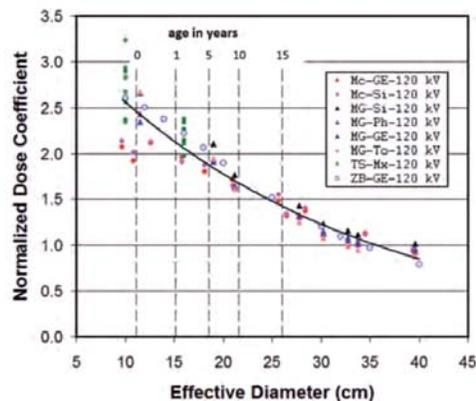
The normalized dose coefficient for the 32 cm PMMA  $CTDI_{vol}$  phantom is shown as a function of effective diameter. The individual data points correspond to four independent research groups, as indicated in the key. (Mc=McCollough, MG=McNitt-Gray, TS=Toth/Strauss, ZB=Zhou/Boone). Scanners represented are also indicated in the key (GE=General Electric, Si=Siemens, Ph=Phillips, To=Toshiba, Mx=Mixed Scanner manufacturers).
