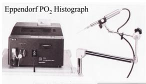
The Au electrode is in a Pt needle. Electrolysis of O<sub>2</sub> gives a current proportional to PO<sub>2</sub>.
