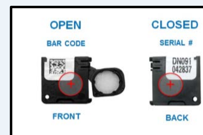
Fig 1. The "open" position was used when annealing and exposed to ambient clinic light (2).
