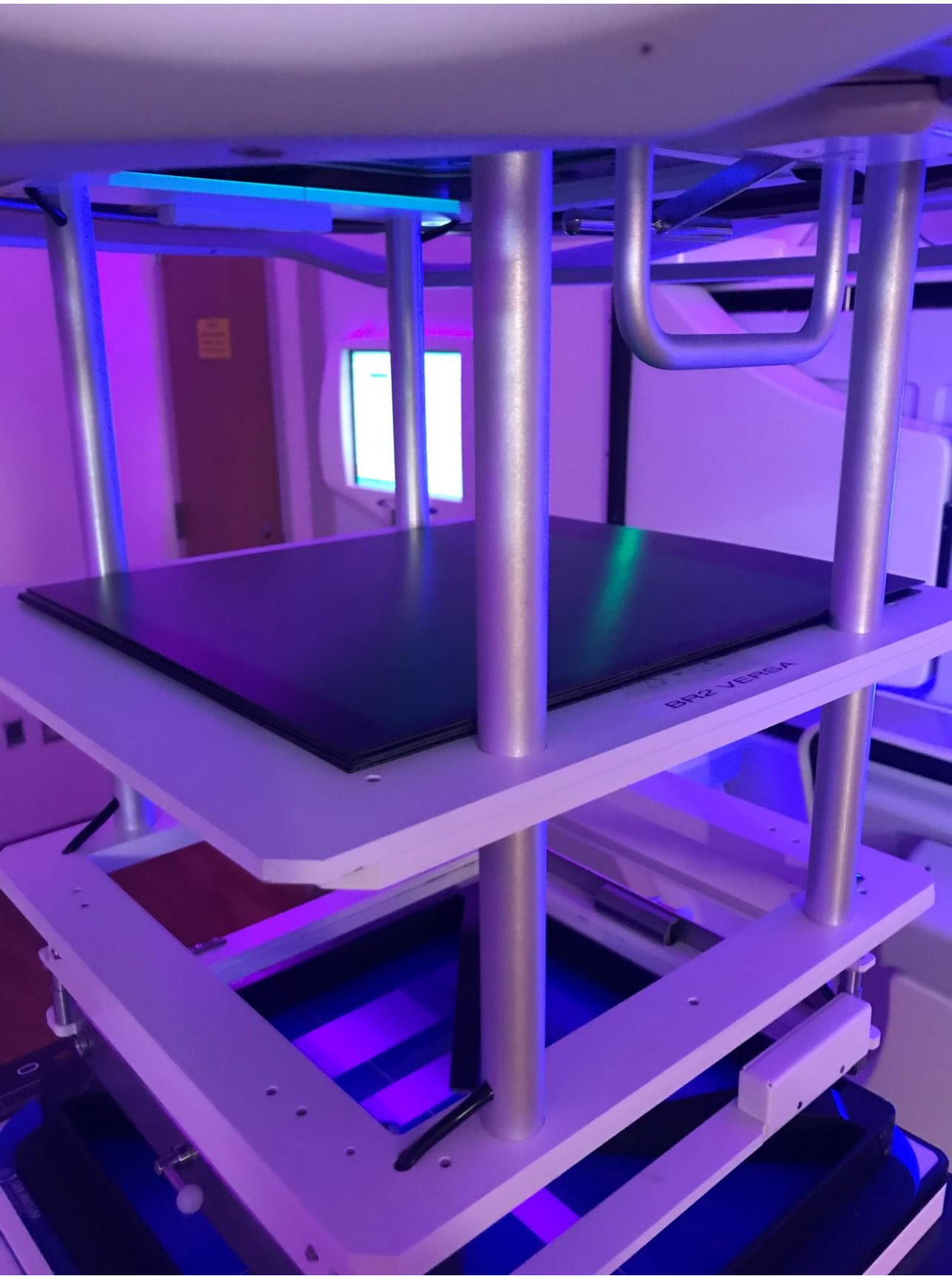
Figure 5. IC-Profiler set to 100cm SSD with Quad Wedge placed on the surface and 5mm of PVC placed in 25cm x 25cm cone
