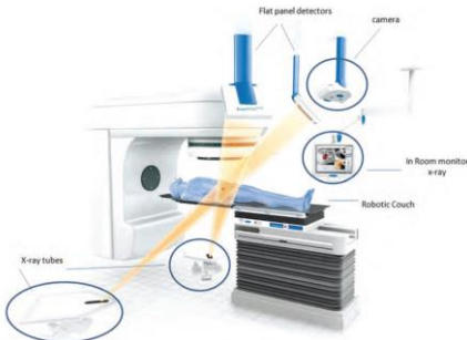
Fig. 3 The Exactrac™ system with floor-mounted x-ray tubes and ceiling-mounted flat panel detectors (from ICRU-91)
