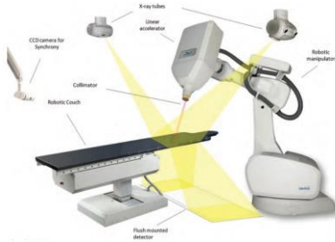
Fig. 2 The CyberKnife™ system with its main components including IGRT systems. The stereotactic x-ray systems have ceiling mounted x-ray tubes and floor-mounted detectors. The x-ray systems are supplemented with a ceiling-mounted camera to determine the patient surface contour. (from ICRU-91)
