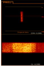
**Right:** Linogram/Cyclogram of the line source projections. No discontinuity observed between the two detector heads.
