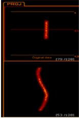
**Left:** Sinogram of the line source projections. No discontinuity observed between the two detector heads.
