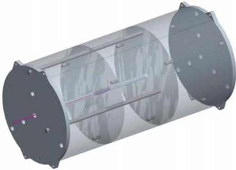
30 cm in diameter by 60 cm in length and is made of high density ( $0.97 \text{ g/cm}^3$ ) polyethylene. There are three sections, 29.3 lb (13.3 kg mass) each. (The 32 cm CTDI phantom has a mass of 14.4 kg.)
