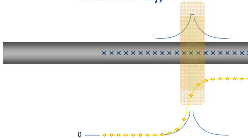
one could perform only one axial exposure with the phantom not moving and measure the dose at points all along the dose profile. Then add all these individual doses together. (In order to make the total come out the same, the distance between the individual dose measurements would be the same as the table movement per rotation of the slide shown earlier.) Alternatively, use a really long skinny ion chamber.
