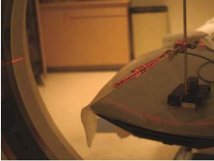
Thimble ionization chamber free-in-air and aligned along the axis of rotation. The chamber is attached to an extender rod from a lab stand, and the assembly is illuminated by the CT system alignment laser lights.
