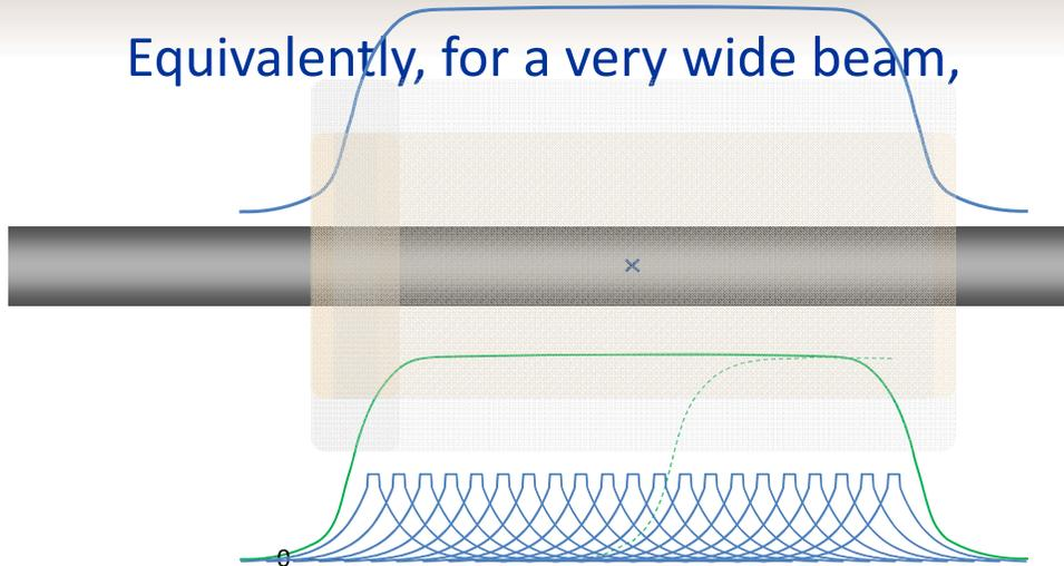
*we could imagine that we have a situation like the original example but with a coordinate change to a fixed table and a moving gantry. Then simply replace the series of narrow beams with a single wide beam and measure the dose at a single point in the center. (The curve has been smoothed.) The dose in the broad flat region is  $D_{eq}$ . Concept of Irradiated Length.*
