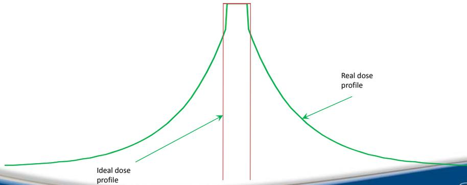
Based on data from TG200 very long phantom measurements.
