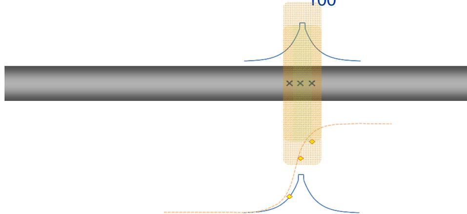
The chamber normally used is 100 mm long. It is not long enough to capture the entire dose profile and leaves off the tails. Thus, as you can see, the cumulative value is less than would be for an infinite scan. When we use a pencil chamber that is too short to capture the entire profile, the CTDI value we get is equivalent to that for a scan that is the length of the chamber. For a 100 mm chamber, we get  $CTDI_{100}$ .
