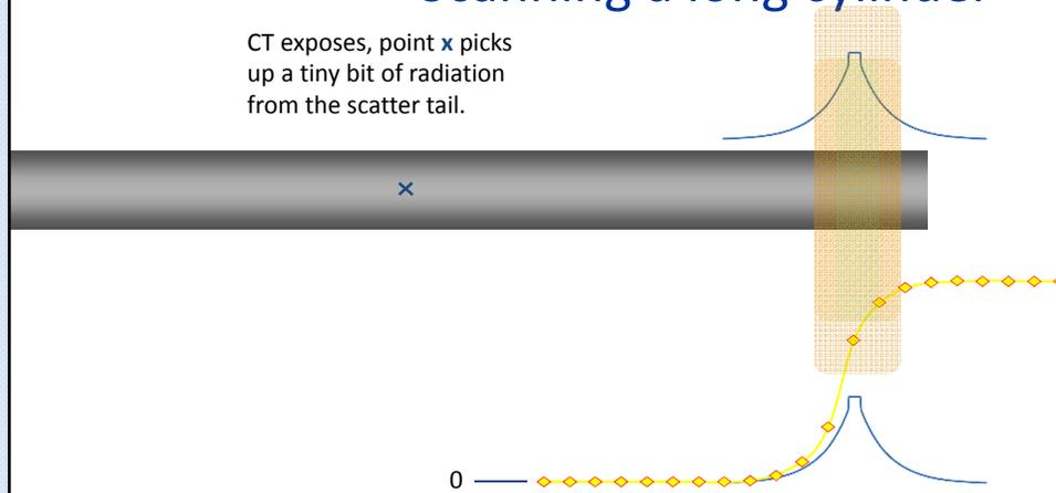
*Note: Note that if the scans are closer together, the ultimate dose will be higher. Although an axial scan is depicted, the extension of the concept to helical scans is obvious.*
