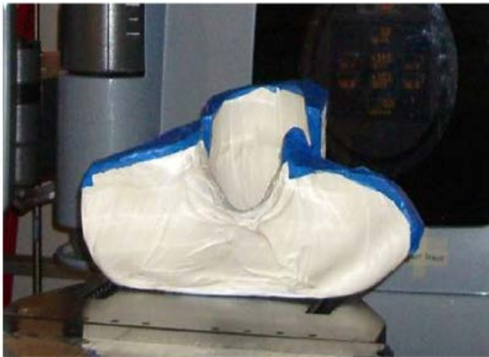
Figure 1 An example of a patient-specific head mold made out of expandable foam that conforms to the patient's head (CDR Systems, Inc, Calgary, Alberta, Canada).
