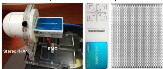
Figure 1: left panel: SMC with StereoPHAN phantom; middle panel: SMC, and right panel: diode array showing the arrangement of the diodes.
