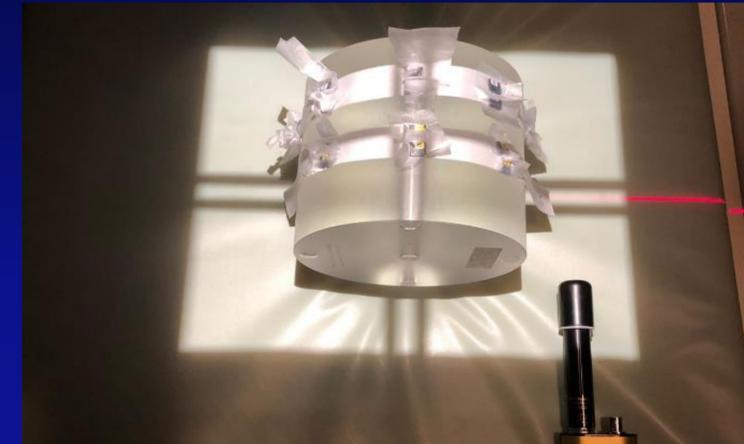
Fig. 4 The new experimental setup viewed from above. Two strips of nanodots on a cylindrical CTDI phantom with a 6 cc ion chamber for exposure consistency monitoring
