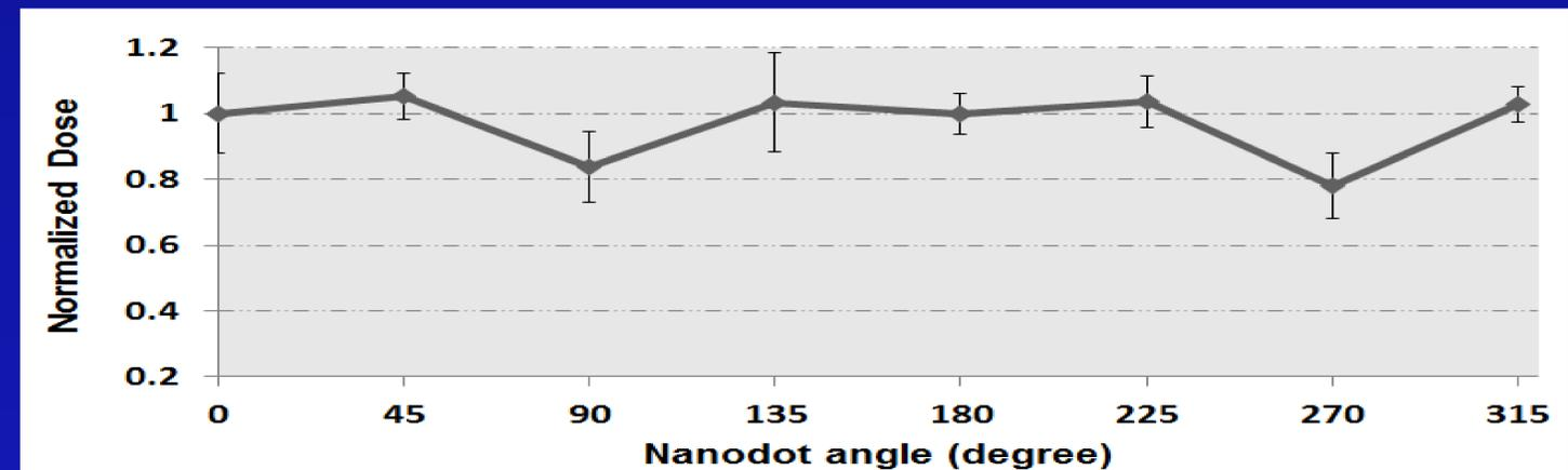
Fig. 5 Dose normalized to 0° versus nanodot angled with respect to the simulated fluoroscopy beam.
