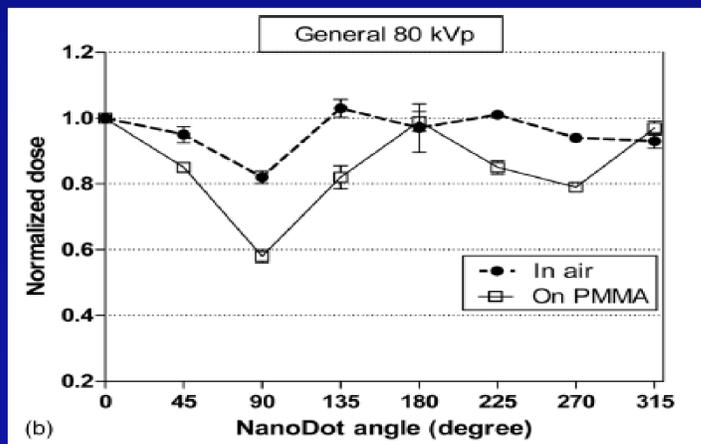
Fig. 1 Results from Al-Senan's characterization of nanodots in general diagnostic energy range from 0-315° at cardinal angles. Dose is normalized to 0°.<sup>1</sup>
