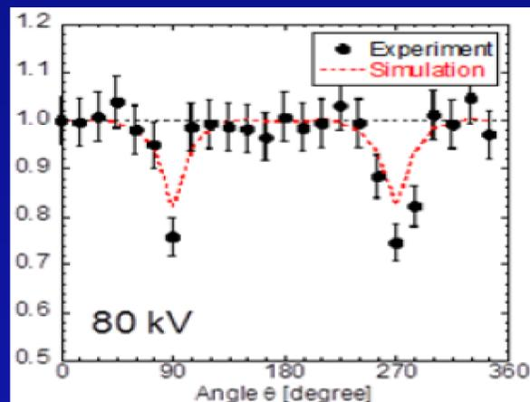
Fig. 2 Results from Okazaki's characterization of nanodots for skin dose measurement from 0-360°.<sup>2</sup>
