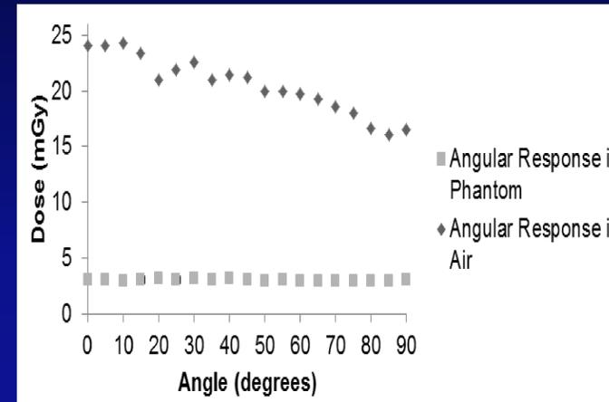
Fig. 3 Previous results in Air and in Phantom showing dose to nanodots with the CT beam angled. Assumed symmetric response.<sup>3</sup>
