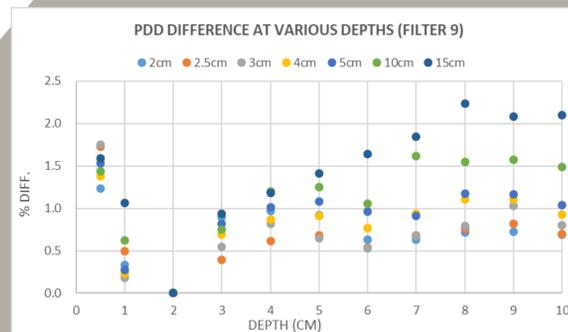
Figure 6 Pdd difference between measurement using Solid water and water phantom at various cone sizes (Filter 9)
