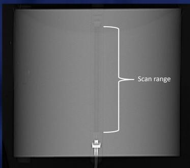
Figure 1. Topogram of the CTDI phantom with pencil chamber inserted. The air volume of the chamber is used to set the scan range.
