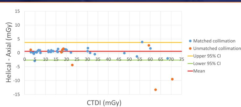
Figure 3. Bland-Altman plot showing differences between the axial and helical measurement methods.
