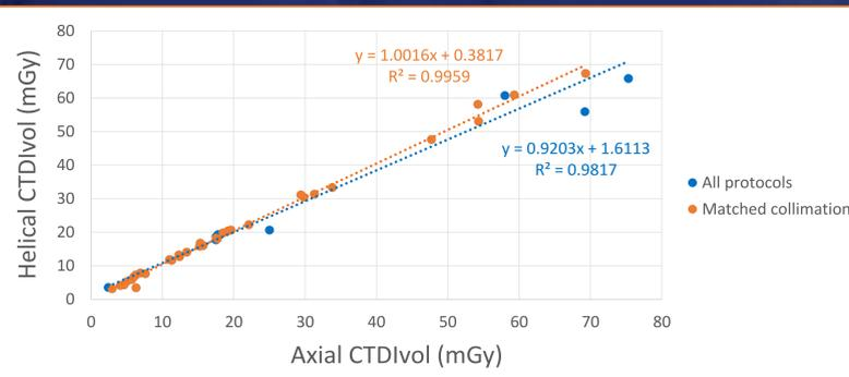
Figure 2. Correlation between axial and helical  $CTDI_{vol}$  values.
