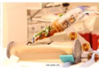
Figure 2B. Coils removed to show phantom, robot, and long thin fiducial in needle guide (cutout in phantom can be seen)
