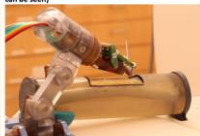
Figure 2D. View from right side illustrating robot mount and simulated positioning between legs
