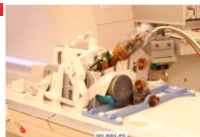
Figure 2A. Robot mounted on table with long bone phantom in middle and imaging coils on both sides
