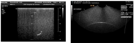
The left half of the array is faulty, with numerous dropout areas.
