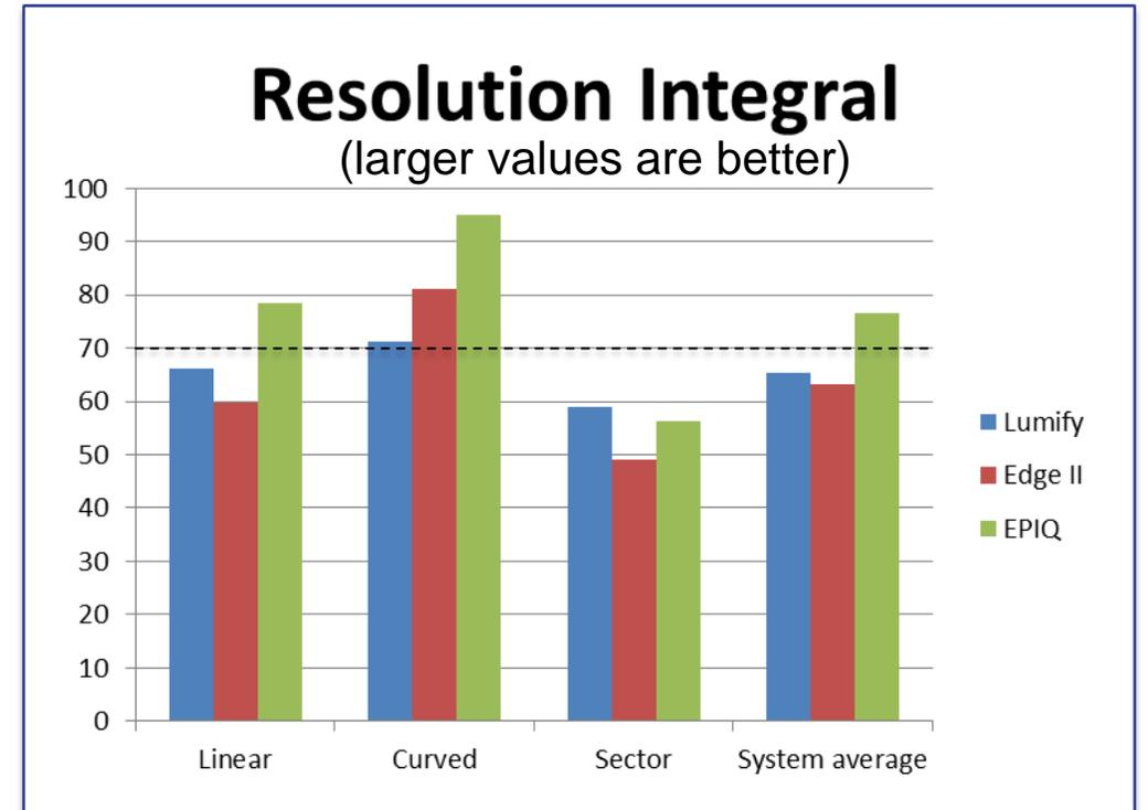
**Resolution integral measurements for tablet-based Philips Lumify, laptop-form factor Sonosite Edge II, and premium Philips EPIQ ultrasound scanners.** A dashed line is shown for  $R=70$ , which is an estimated general reference performance level for systems tested between 2015 and 2019 (extrapolated from Pye and Ellis, Journal of Physics, 2011)
