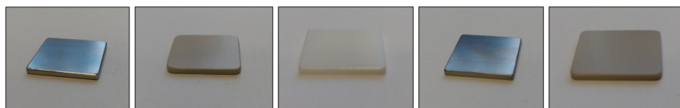
Fig 1. Titanium (1.a), Pektton (1.b), Zirconium (1.c), Cobalt Chromium(1.d) and Peek (1.e) dental specimens.
