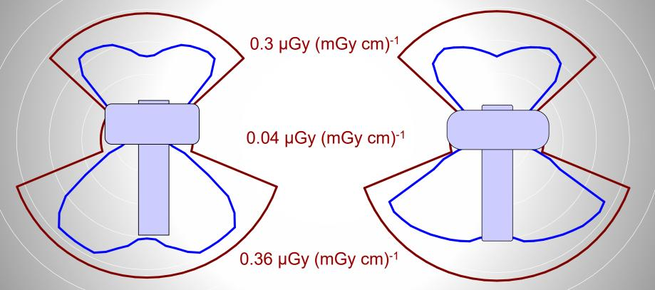
Calculated contours --- are compared with measurements of scatter air kerma ----.
