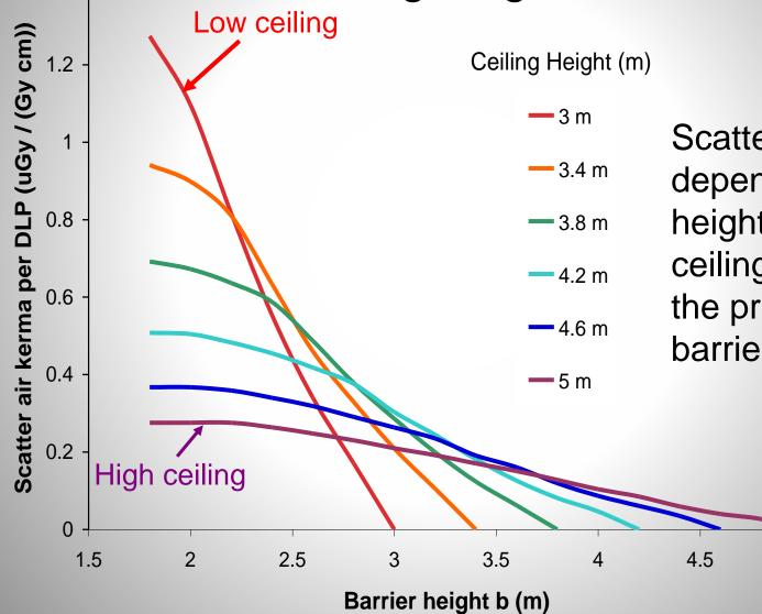
Scatter level depends on the heights of the ceiling slab and the protective barrier
