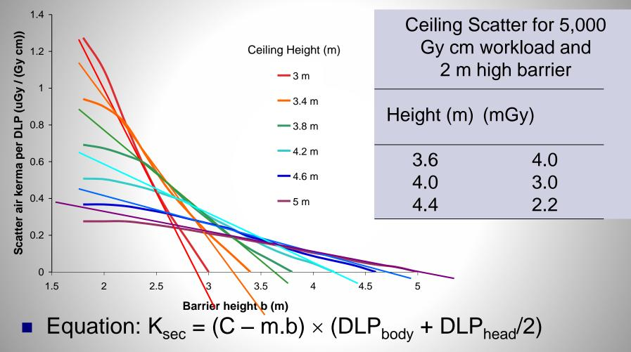
Where b is the height of the barrier and C and m are constants dependent on the height of the ceiling.
