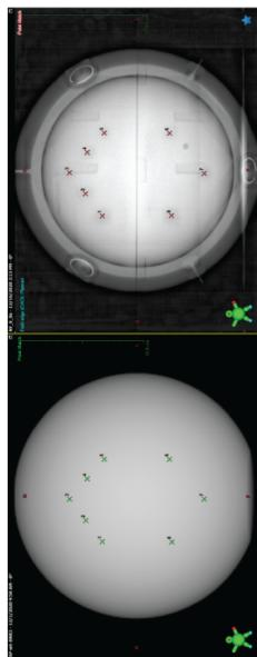
Figure 1: Example of kV image registration based on correlated points in Aria.
