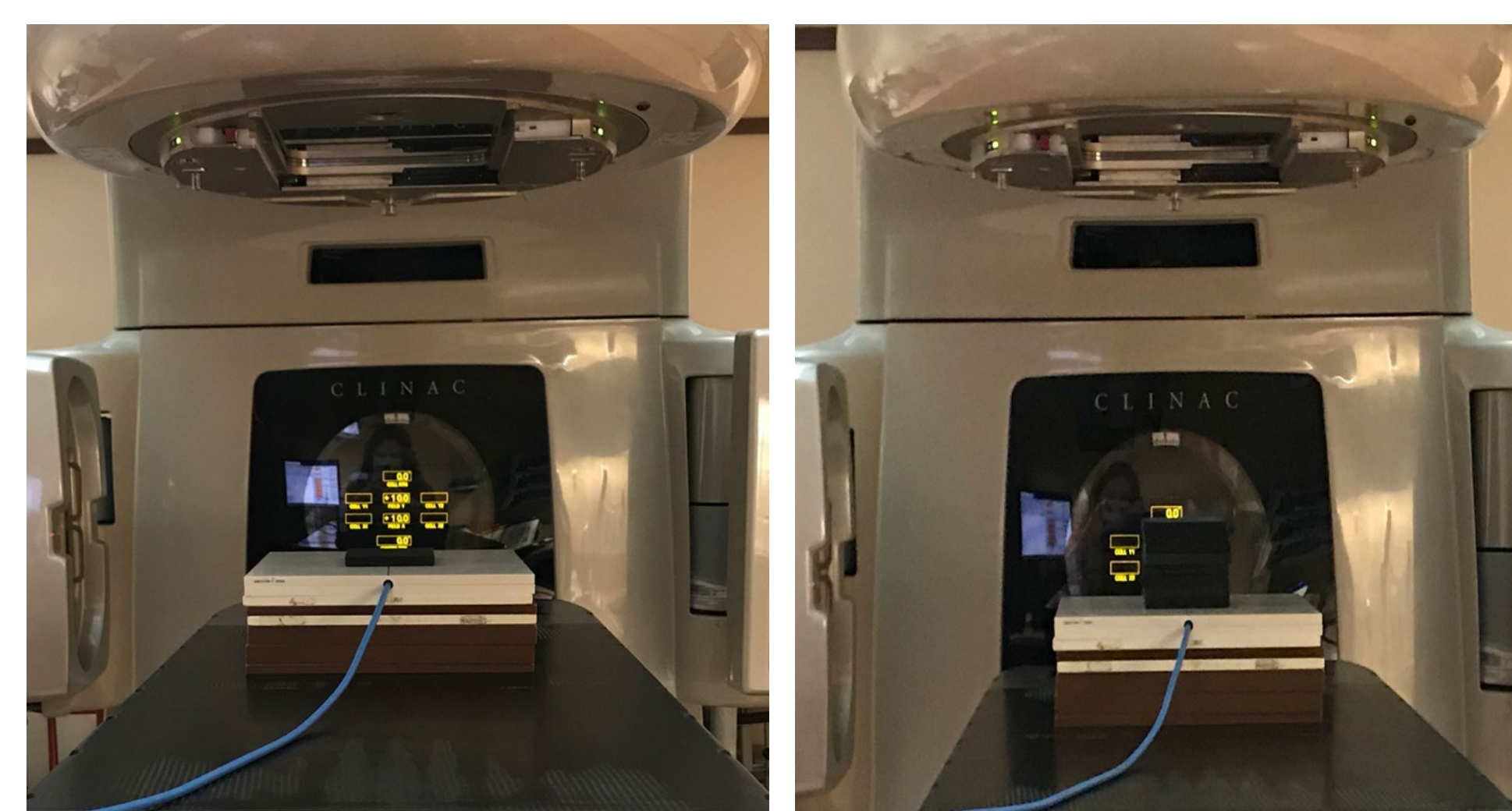
Figure 2: Photon measurements: gantry 0°, collimator 0°, SAD 100 cm, 10x10 cm 2 field size, 1 cm block added after each measurement
