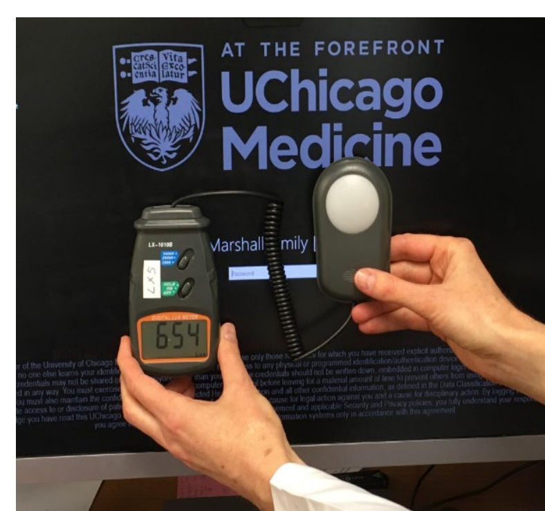
Figure 1. Example of measuring ambient light with an inexpensive photometer calibrated with an in-house photometer with NIST-traceable calibration.
