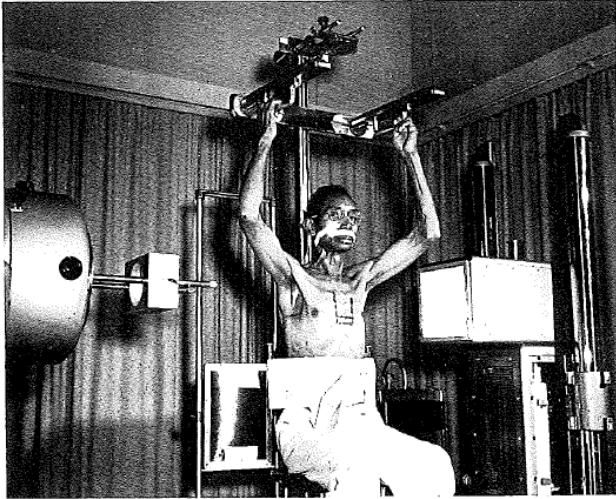
FIG. 1. The target room. From left to right: the collimating device of the 2 mev. Van de Graaff accelerator, the patient in the rotating chair, and the fluorescent screen, orthicon, and signal amplifier.
