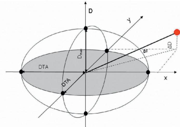
**Fig. 3.** The concept of gamma verification [5]: x, y, D – spatial and dose dimensions; DTA – distance-to-agreement;  $D_{\max}$  – max dose deviation;  $\Delta r$ ,  $\Delta D$  – local spatial and dose divergence of the analyzed point
