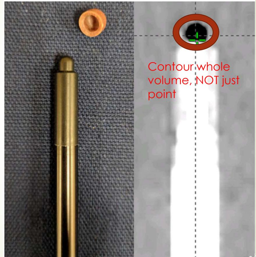
Exradin A26 micro chamber (left) and CT scan of chamber in phantom (right)
