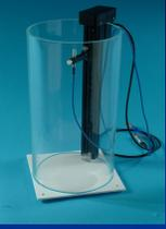
Moving Tank System for TMR
