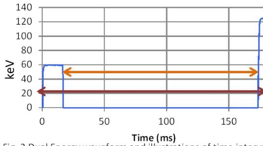
Fig. 2 Dual Energy waveform and illustrations of time interval and total exposure time.
