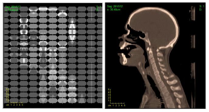
Right: Perfect Registration, Left: Gridded MirrorScope – Notice that each circular region within the grid is symmetric about the vertical axis.
