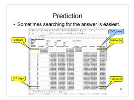
One cannot easily calculate the release time analytically for the more complicated models. A straightforward approach is to develop a spreadsheet that tabulates the doses on out to infinity for various release times. One them simply searches through the table to find the release time at which the dose has fallen to the desired level. Another approach is to use the calculators on the RADAR Web site and adjust the release time until
