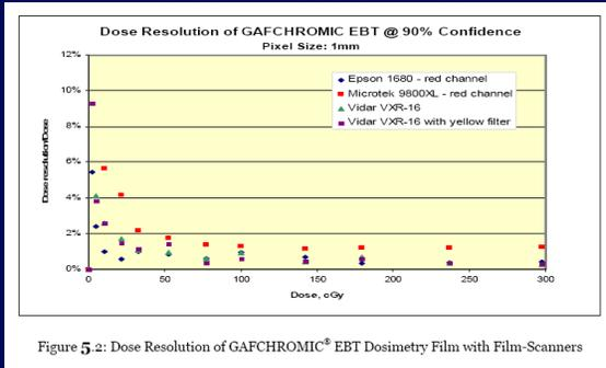
Figure 5.2: Dose Resolution of GAFCHROMIC® EBT Dosimetry Film with Film-Scanners
