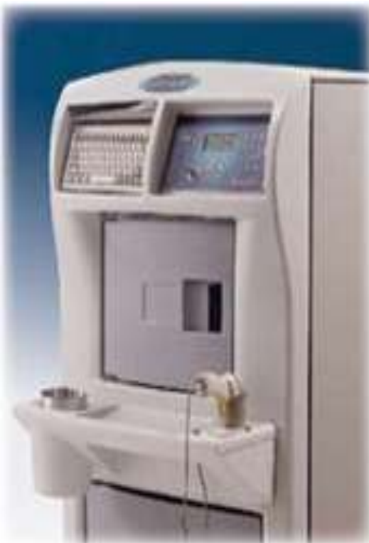
Gammacell® Irradiator 1000 Elite / 3000 Elan ~ 750 Ci to 3000 Ci Cs-137
