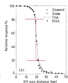
Off axis profiles at the isocentre (FAD D 100 cm), 6 cm deep, measured with diamond, shielded diode, and radiographic film and calculated using MC (EGS4), for (a) 7 mm and (b) 23 mm SRS collimators.
