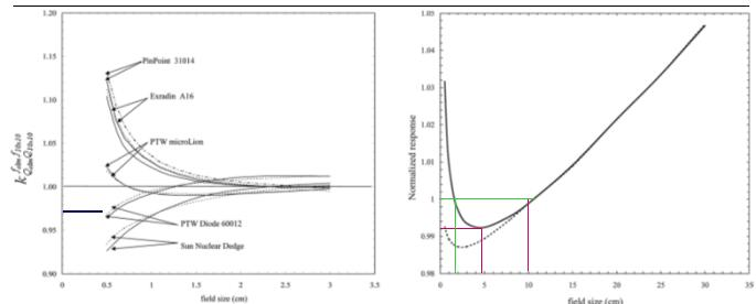
FIG. 7. Correction factor  $k_{Q_{det},Q_{beam}}^{F_{beam},F_{det}}$  for five detectors as a function of the field size, for 6 MV beams of Siemens (dotted line) and Elekta (continuous line) linacs.
