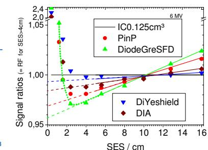
FIG. 3. Detector signals relative to the reference ionization chamber signal  $[D_{\text{det}}(s)/D_{\text{IC}}(s)]$ . The factors for  $\text{SES}=8$  and  $4\text{ mm}$  are not shown. They are in the range of 1.3 and 2.3 respectively. Solid lines: linear regression of  $k_E(s)$  for  $s = \text{SES} > 5\text{ cm}$ , dashed lines: extrapolation for smaller field sizes.
