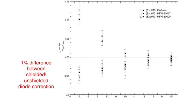
FIG. 6. Measured  $k_{\text{fcln,fmsr}} / Q_{\text{lin}} / Q_{\text{msr}}$  correction factors for 800 mm SSD plotted as a function of iris collimator size for the PinPoint 31014 microchamber, PTW-60017 unshielded, and PTW-60008 shielded diodes. Corresponding results calculated using MC simulation by Francescon et al. (Ref. 37) are plotted for comparison. The uncertainty, at 68% confidence level, of the presented correction factor results are depicted using error bars.
