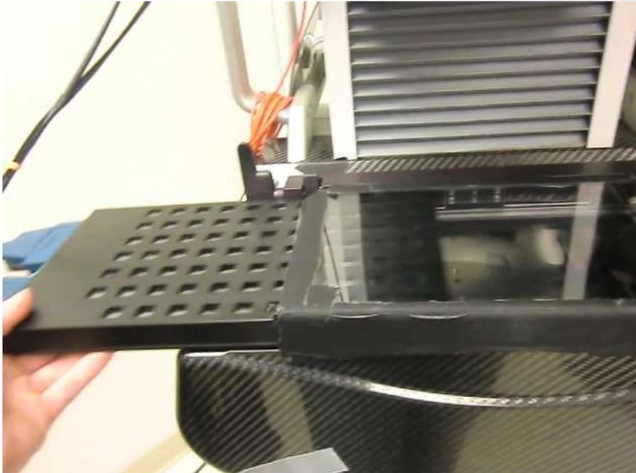
Detector panel can be easily slid underneath the breast before the patient arrives and then removed in a couple of seconds prior to the X-ray imaging. This detector cover was designed in conjunction with Hologic to maintain clinical quality dbt scans.
