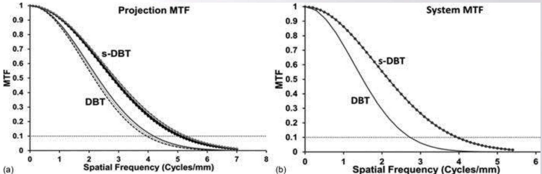
(a) The projection MTFs of the stationary and rotating gantry DBT systems along the scanning direction. (b) The system MTF obtained using reconstructed in-focus slice.
