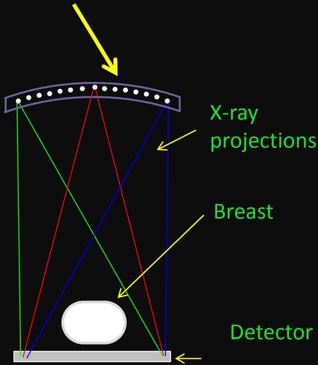
Multiple stationary sources with a main high power x-ray source
