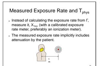
To adopt a bit more realism, the exposure rate at a meter is measured, but the radioactivity in the patient is still assumed to disappear only by physical decay. While this ignores biological clearance and it treats the exposed person as a point target, it does take into account attenuation by the patient's body.
