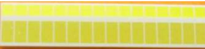
Stacking Dual-Layer 1-D arrays into a single standard detection tile
