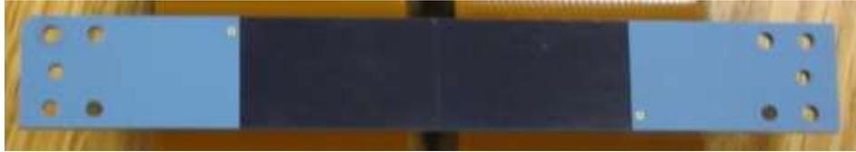
Back illuminated "64 slices" photodiode "flip-chipped" to a substrate
