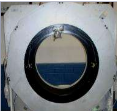
Ingenuity TF PET/MR Gantry with laminated steel shield
