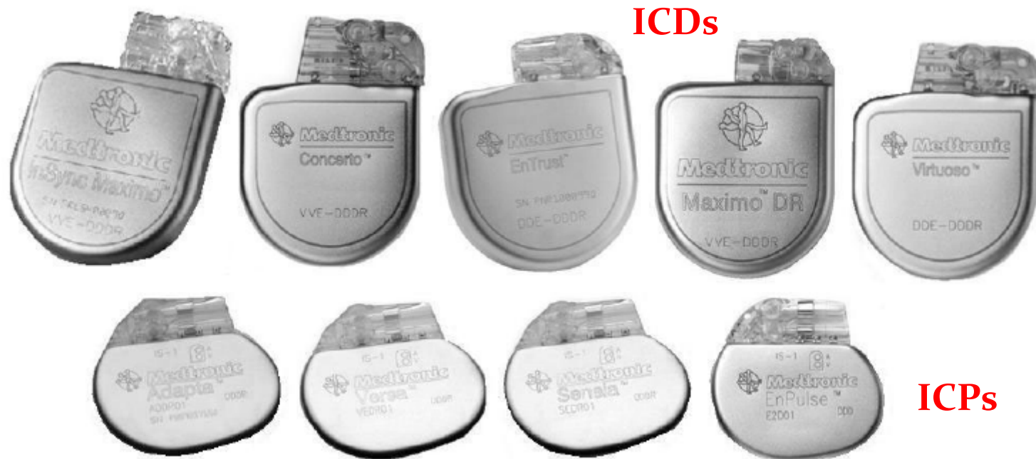
FIG. 3. [Top]: Five ICDs [Left to Right]: InSync Maximo model 7304, Concerto model C154DWK (VVE-DDDR), Entrust model D154ATG, Maximo DR model 7278, and Virtuoso model D154AWG; [Below]: four implantable pacemakers: Adapta model ADDR01, Versa model VEDR01, Sensia model SEDR01, and EnPulse2 model E2DR01.
