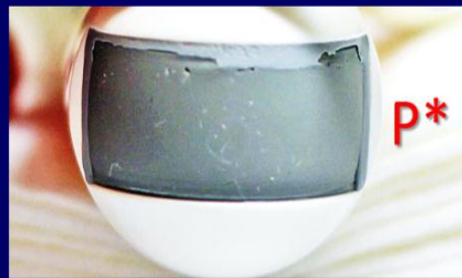
Lens Peeling / Delamination
