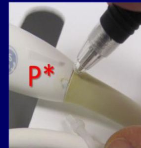
Peeling of Housing Layer
