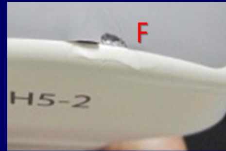
Cracked Housing/ Lens Damage
