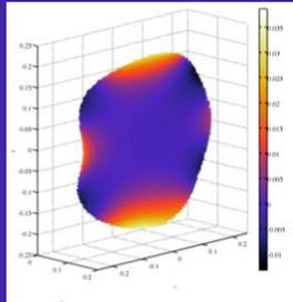
Slice distortion in experimental system, 10cm off-centre slice in 50cm DSV (all quantities in metres)
