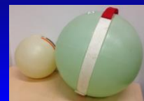
Spherical phantoms –17 cm and –26 cm
