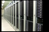
Dedicated data system filters to 100,000/s (L1), 3000/s (L2), 200/s (L3) – for detailed analysis
