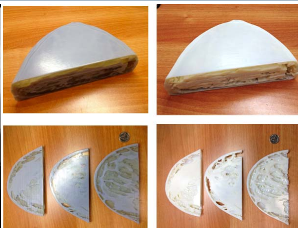
Fabricated (3D printed) physical breast phantoms, the Doublet (left) with two materials and the empty Singlet (right) with a single material, both in three slabs of 15 mm each.
